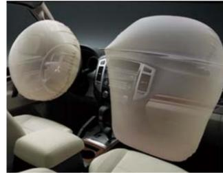
Driver's and front passenger's front SRS airbags (dual-stage) 📷 03
