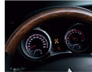
High-contrast back-lit meters and gauges with tachometer, 4WD position display and rheostat 📷 22
