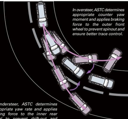
In oversteer, ASTC determines appropriate counter yaw moment and applies braking force to the outer front wheel to prevent spinout and ensure better trace control.
